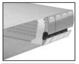
2. Pull the handle out to unlock the canister from the **FORTRA®** unit. Ensure that the thumb is placed below the line. Pressing the thumb against the Status LED lens could break it. Notice that the locking tab slides down as the handle is pulled out.
